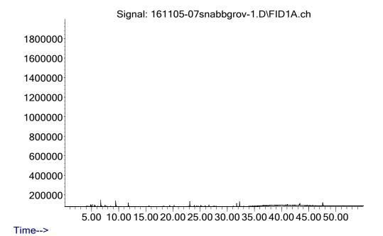
TVOC between  $C_6$  and  $C_{16}$ , means compounds eluting between 6.2 and 37.9 minutes.
